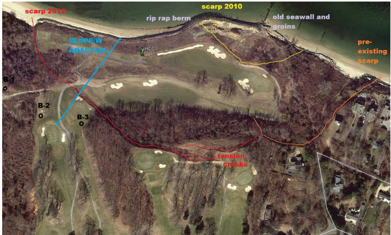
Figure 1. Google Earth Photograph Circa 2012 with Interpreted Landslide Scarps, Tension Cracks, Approximate Boring Locations, and Presumed Slope Stability Profile Location
